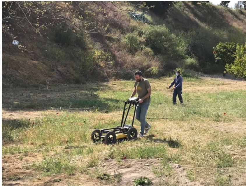
Figure 10. Subsurface survey with ground-penetrating radar
